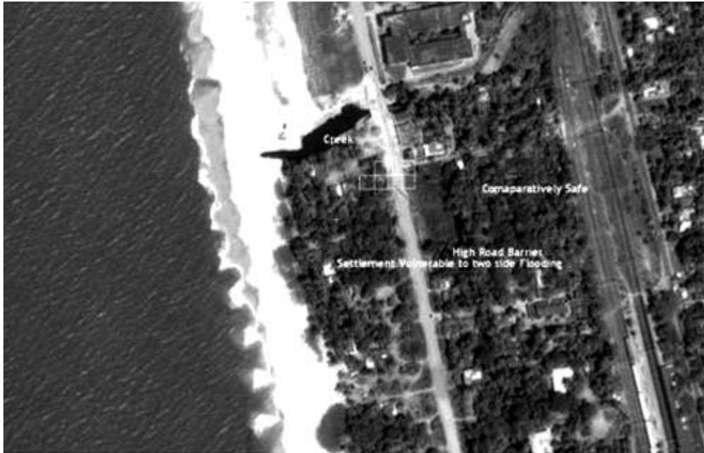
**Figure 3. Settlement vulnerability mapping using QuickBird image of 0.6m spatial resolution.**
