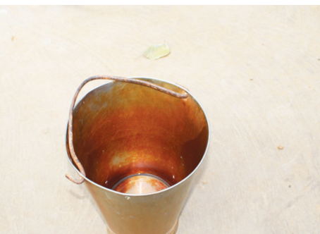
Figure 8 : Rust due to poor quality of water
