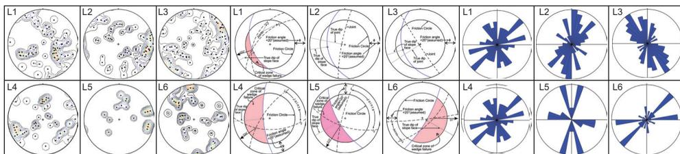
Results from Stereographic projection and Rose diagram generated from the joints of the study area:
