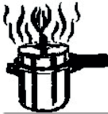
Safety valve releases pressure
