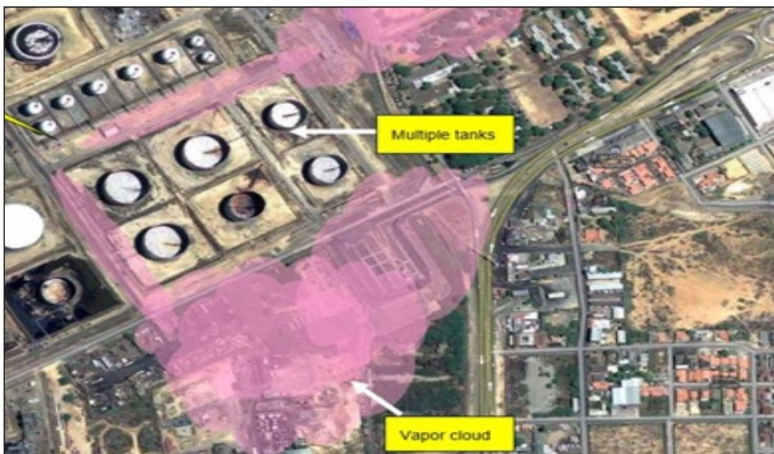
Figure 7 Unconfined vapor Cloud Explosion in a Refinery Complex, Venezuela
