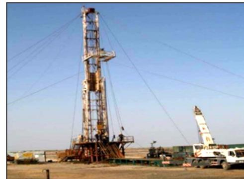
Figure 12 An example of Work-Over Rigs
