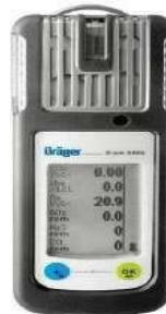
Figure 81 Multi-gas detector
