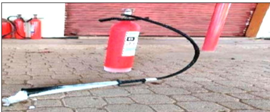
Figure 15 Dry Ice formation from discharge horn
