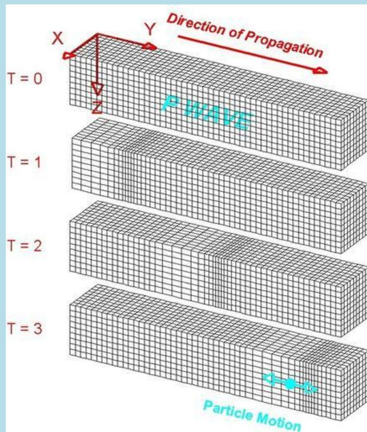
**A P wave travels through a medium by means of compression and dilation. Particles are represented by cubes in this model.** *Image ©2000-2006 Lawrence Braile*
