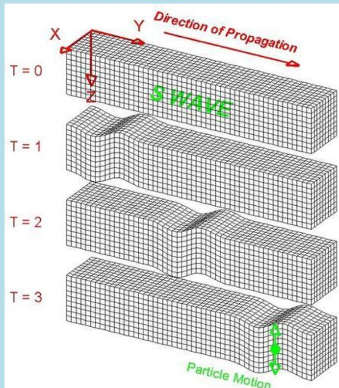
**An S wave travels through a medium. Particles are represented by cubes in this model.** *Image*
