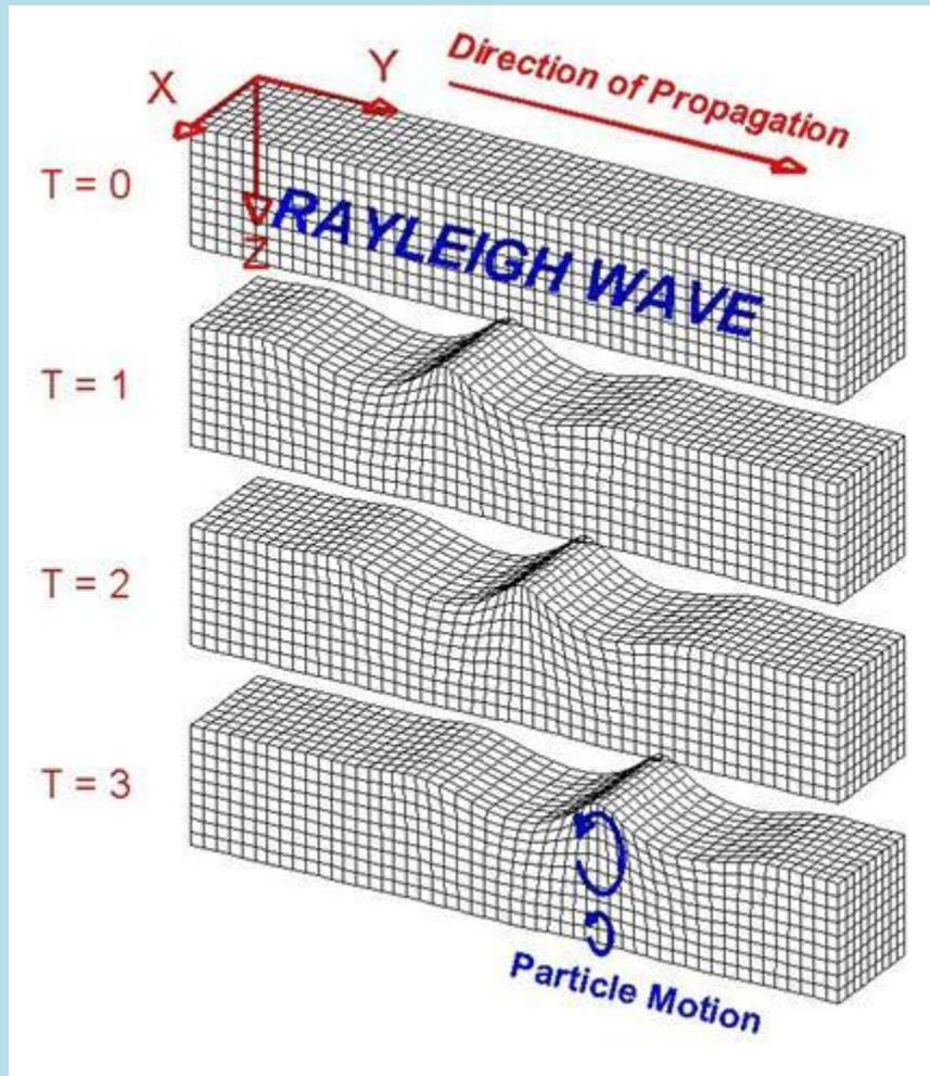
A Rayleigh wave travels through a medium. Particles are represented by cubes in this model. *Image ©2000-2006 Lawrence B*
