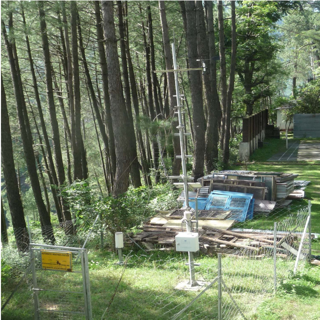
Fig 1.63: Automated Weather Station for recording rainfall, temperature and pressure at DGBR office, Tekhla
