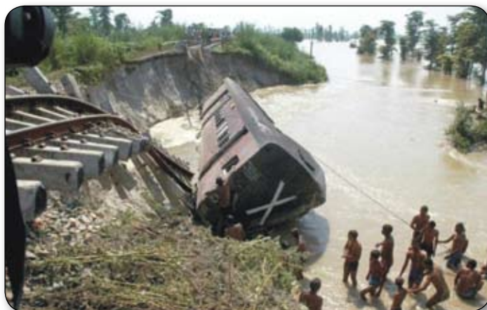
Railway workers engaged in rescue operation after the railway tracks gave way causing a rail car to fall off the tracks in floods near Kasganj, UP.
